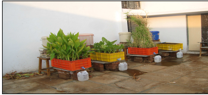
Figure 2: Experimental Setup of Constructed Wetland
